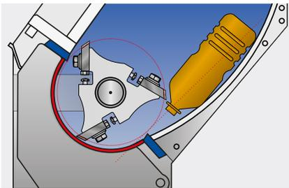
The strongly curved, tangential back wall of the cutting chamber, combined with the aggressive open rotor design, ensures reliable material in-feed and minimises the risk of bridging in the hopper.
