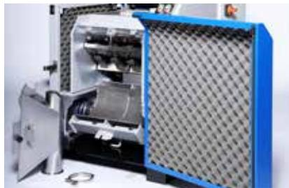
The granulator stands out for its easy accessibility for cleaning and maintenance, making it especially service-friendly.
